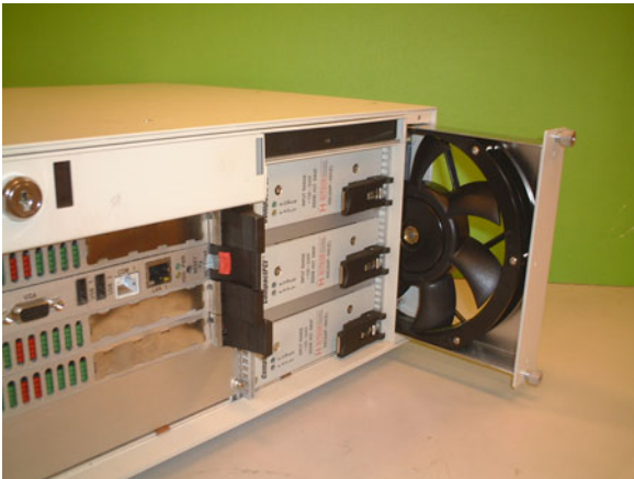
Figure 2.8: Hot-swappable fan maintenance
